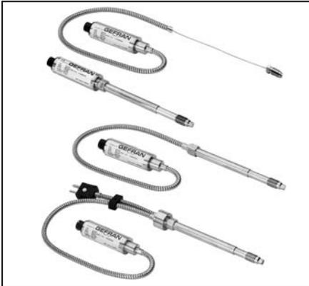
The M, W and K series melt pressure transducers and transmitters measure pressure in high temperature locations by hydraulic transmission of the pressure signal to a strain gauge element.
